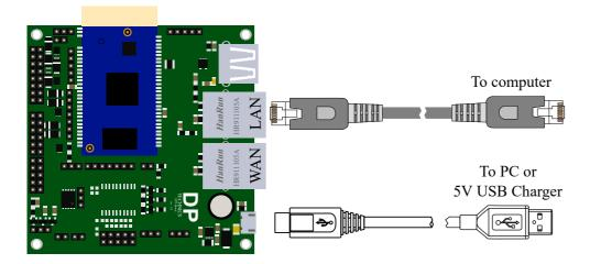
It is perfectly normal that the DPT-Board ethernet connector LEDs will not turn on. We have opted to give the user more available GPIO pins instead of using 4 GPIOs to drive the ethernet connector LEDs. The connection is successful when your computer gets an IP address assigned by the DPT-Board.
