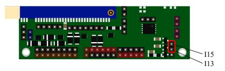
The inputs are pull-up by default and you can make them low by connecting to ground. The high voltage inputs are protected by BAT54S diodes and an RC-circuit. This means the **absolute**maximum input voltage is 30V. The RC-circuit protects against spikes when the input frequency is high.
