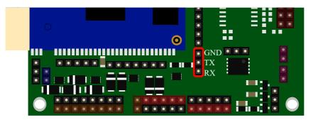
The bootloader and Linux image will both talk via the serial port, the linux talk however can be turned off. The communication settings to read the info on the serial port are the following:
