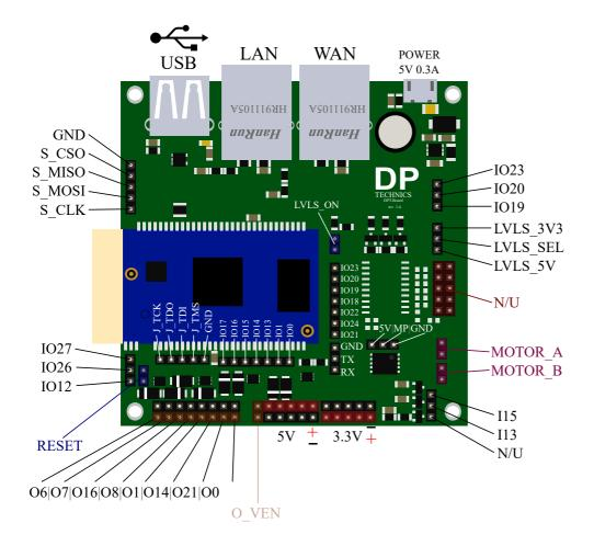
The following connections are available on the DPT-Board model.  $\ensuremath{\text{N/U}}$  means the pins are not used in the current version.
