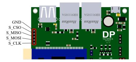
The **S\_CSO** pin is actually the chip select used for the internal SPI flash. This active-low pin can be used by external circuitry to check for flash disk activity. When you use the hardware SPI port for another peripheral **GPIO26** is the chip select for the second device. You can off course also use another GPIO and control it separately.
