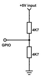
This provides a simple way to interface with 3V3/5V logic on every GPIO pin. Off course you can also use the DPT-Board's high voltage inputs or level-shifted GPIO's if you want to interface bidirectional communication busses such as 1-Wire and I2C. You can find more information under the designated paragraphs.
