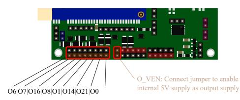
The GPIO's shown in the drawing above are equipped with a high power MOSFET (MCH6662) and a protection diode (S1A). This enables them to switch high current inductive loads. The **O\_VEN** can be connected with a jumper if the internal 5V supply must be used to drive the loads connected to the high power outputs.
